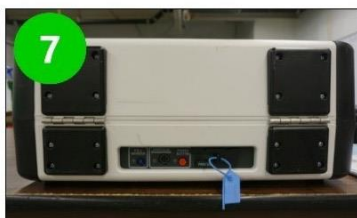
Blue Security Seals from Printer Port on TouchWriter (rear near power button). Removed when setting up.
